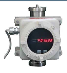
This instrument has been designed to measure the instantaneous and total flow of fluids, approved for use in areas with danger of explosion. It allows instant reading of the product flow rate in It / h, reading of the totalization of the product flowed from a certain instant in liters or in hectoliters, the setting of the threshold in liters or hectoliters of the product to be measured, the sum of the partial counts of the fluid product.
